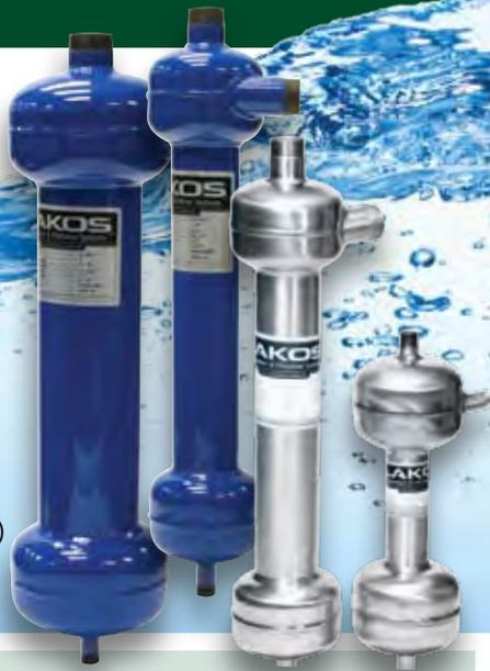
The ILB/ILS offers the benefits of high pressure capabilities and much higher temperature resistance. Heavy duty construction typically withstands even the toughest environmental conditions. Available in carbon and stainless steel. The ILB/ILS centrifugally separates up to 98% of particles 200 mesh (74 microns). Innovative patented design. No moving parts to wear out or replace. Low and steady pressure loss. No routine maintenance. Minimal water loss.
